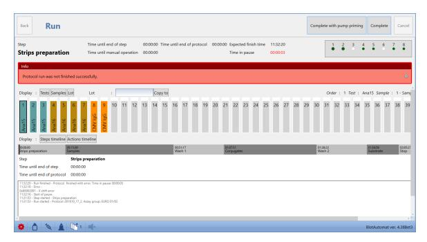
**Stopping the run** - at any time the user can press the "Cancel" button. The system definitively ends the run - this ending is irreversible. The time of stopping is entered in the protocol and the protocol is assigned a status of "Not processed - error".
