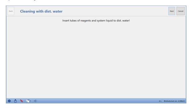
The user inserts system the system solution and reagent pump tubing into a bottle with DI water. By pressing "Next" the system flush the tubes.
