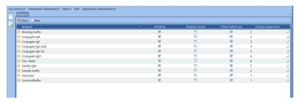
For each edited reagent there are attributes "Antidrop", "Reagent saving", "Prime before run" a "Pumps assignment", which make the work with reagents more accurate during sample testing.
