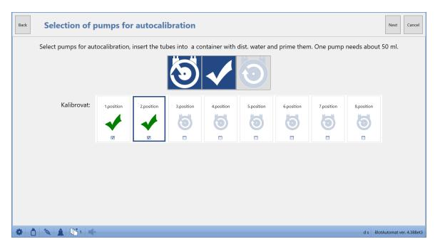
To perform autocalibration the user selects the pump, which he wants to calibrate. Then he inserts the tubing of the selected pump(s) into a bottle with DI water and then select the pump with the
