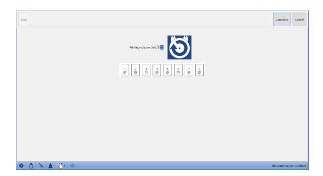
The user puts the reagent tubing to the bottle with destilled water. The button cleaning pump by pump. The cleaning can be arbitrarily repeated.
