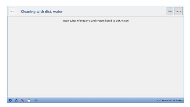
The user inserts system the system solution and reagent pump tubing into a bottle with DI water. By pressing "Next" the system flush the tubes.
