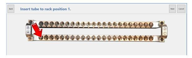
The user inserts the tube into the position marked by the arrow (standard - position 1, control - position "A" ).
