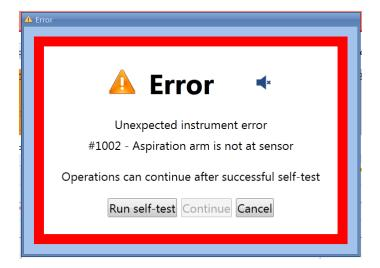
In relation to the mistake type the system offers the user solution options. If the user chooses the self-test, which then runs successfully, it is possible to continue in the interrupted run.
