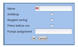
If the user entered all items of the new reagent, he presses the "**OK**" button and the system will save the new reagent in the list. After pressing "**Cancel**" the window for entering new reagents will be closed.
