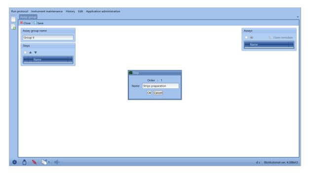
If he has selected a row with the step and presses the the "**Open template**" button in the upper right corner of the application, he can create a new step from the individual actions.By dragging the step
