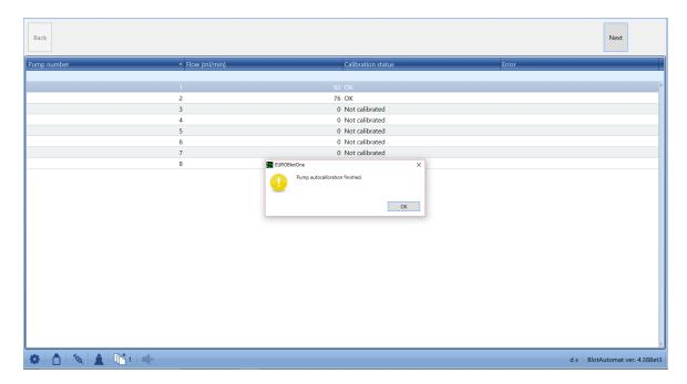
If the autocalibration is error-free and the value of the given pump is found in the requested range the pump status is set to " $\mathbf{OK}$ ".
