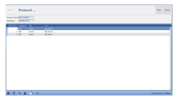
**If the instrument uses the bar code reader** and the user requests to continue with the protocol, he presses the "**Next**" button and the system displays a prompt to insert the sample rack into the instrument with a query to continue with the sample scanning.
