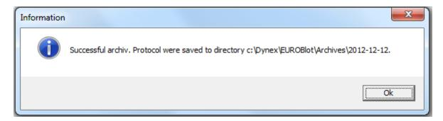
The system creates an archive file with the appropriate protocols in the XML format, which are then saved into a folder e.g. "2012-10-26" with path: c:\Dynex\EUROBlot\Archives\2012-10-26. The folder created for storage of archived protocols is named after the date of archive creation in the format Year (4)-Month(2)-Day(2). The user can view the archived protocols outside the application with an internet browser.
