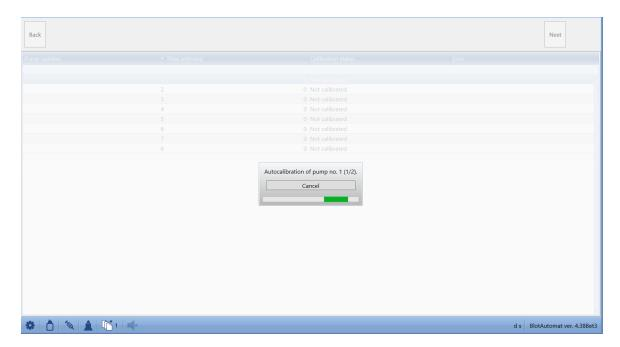
The process itself proceeds individually for each pump. The first required pump starts filling the cuvette until it's full and the tip signals that the level of primed liquid has been reached. The liquid is then pumped into the waste bottle.
