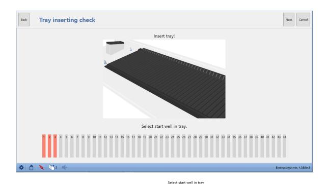
By clicking into the strip field he can to select the starting position, from which the sample testing will begin (in case that a previously partially used tray is inserted). The user may select only such starting position, which is followed by a sufficient number of empty wells for all sample tests.
