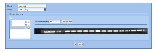
The instrument will move the arm with the camera above the first well in the strip tray. The system displays a window with the real camera view, the user can the move the time slider of the shutter and select the slider position with the best display of the actual camera view. This way he sets the shutter time.
