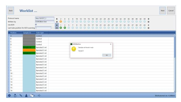
If the instrument does not use the bar code reader - the system fills the sample IDs into the worklist according to the imported protocol. The user inserts tubes with samples into the rack according to the positions in the worklist. If it isn't possible, the user ends the editing of the imported protocol by pressing "Cancel", because the sample ID cannot be edited.
