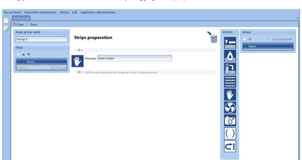
After creating an assay group the user creates individual assays by pressing icon in windows Assays. The asssays can differ in parameters of some operations - volumes and types of reagents for dispensing and the volume for sample pipetting. The change is made by selecting the required assay and then selecting the activities in the step, where the change of parameters is required. These assays will be offered to be assigned with tests.
