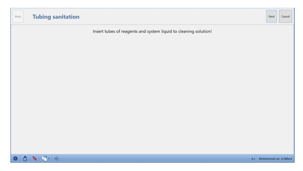
The user inserts the system solution and reagent pump tubing into a bottle with the cleaning solution. By pressing the "Next" button the system flushes tubes with a cleaning solution. The volume for the flush is set by *Pumps cleaning volume* in the menu *Application administration / Settings*.
