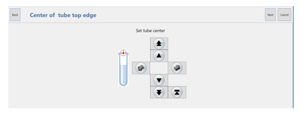
By pressing the control arrows the user moves the lower end of the needle above the center of the upper edge of the tube. This point is the start point for the level detection before the loading of the sample.
