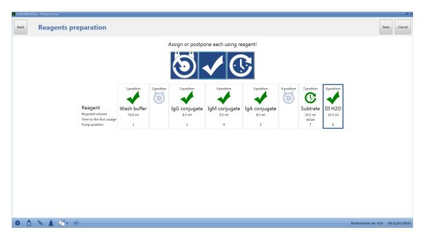
If the user confirmed the loading of all necessary reagents (or postponed it), he can continue with the processing
