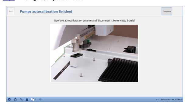
If the system performed autocalibration of the selected pumps, the user removes the cuvette from the instrument and disconnects it from the waste bottle.
