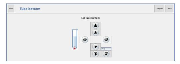
By pressing the control arrows the user moves the tip just above the bottom of the tube. This point is final for the sample level detection.
