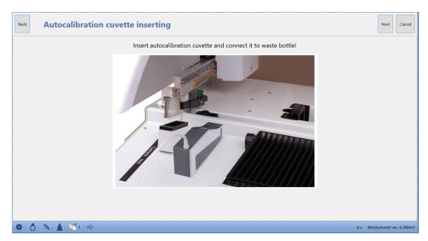
The user places the calibration cuvette on the upper case of the instrument according to the picture and connects the cuvette tube to the waste bottle with a self-closing clutch.
