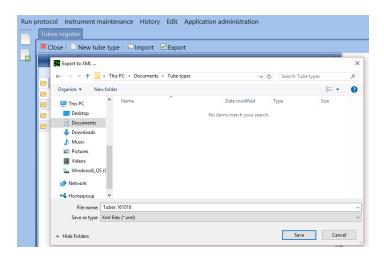
The system displays a Windows Explorer window, where the user selects a location to save the file with exported tube types. He selects the file name and click on the "Save" button. The system saves all tube types, registered in the application, in an XML file. The exported file can be imported into an application located at a different place.
