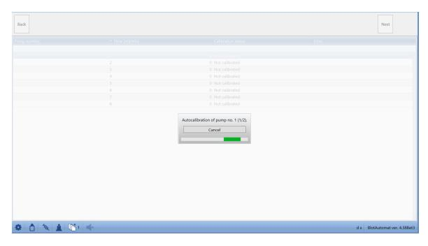
The process itself proceeds individually for each pump. The first required pump starts filling the cuvette until it's full and the tip signals that the level of primed liquid has been reached. The liquid is then pumped into the waste bottle.
