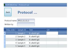
**Sample test lot** - by clicking into the field "**Lot**" the user may assign a lot number to the test or he may let the entry of the lot to the instrument run itself. (see step 7 - Instrument run).
