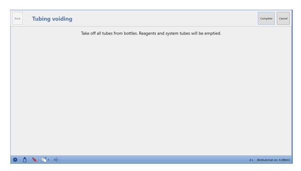
The user takes out the reagent and system solution pump tubing from the bottle and continues to complete the weekly maintenance by pressing "Complete". The system empties the tubes so that there won't be any remaining liquid. By pressing "Cancel" the user may cancel the weekly maintenance process.
