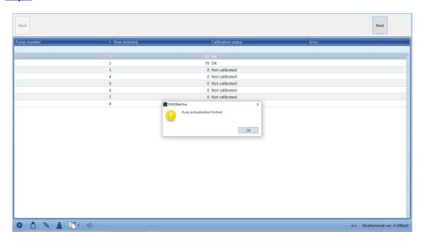
If the autocalibration is error-free and the value of the given pump is found in the requested range the pump status is set to " $\mathbf{OK}$ ".
