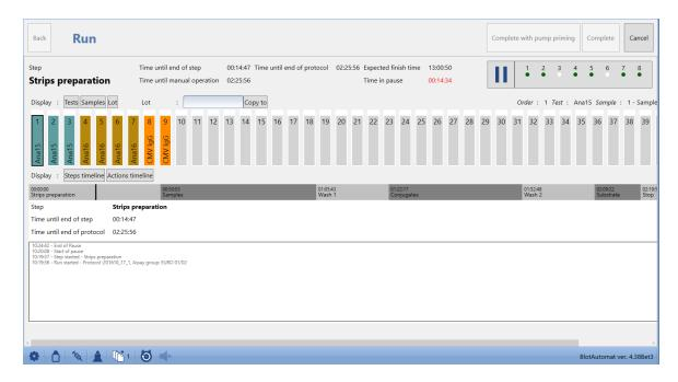
The log of a protocol run is recorded and on-line view is displayed bellow the time line. Log contains the protocol name and time marked records of steps, pauses and errors.
