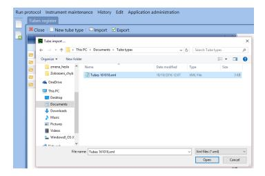
System displays the Windows Explorer window to select an XML file with the exported tube types. The user selects "Open" and the system imports the data from the file as records of tube types. The system then informs about the success of the importing. If it isn't possible to carry out the import, the systems alert the user. The reason may be a damaged file or an incorrect file format.
