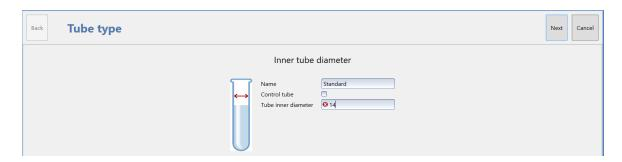
The user enters the **Name** of the tube type (text field) and selects whether this is a **Control tube** type. The user measures the tube for **Tube inner diameter** (in millimeters). This value is necessary for the correct function of the level following during sample taking.
